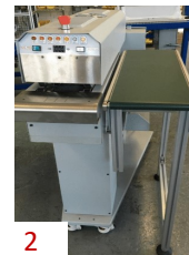
Conventional conveyor powered or unpowered extension tables to support long heavy harness
