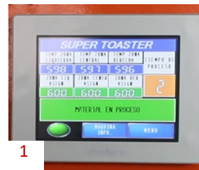
1 5.7 "touch screen independent of the control box for better use of the work area
