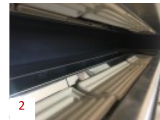
2 Triple heat zones with independent temperature on each one to achieve a uniform temperature through the three heat zones
